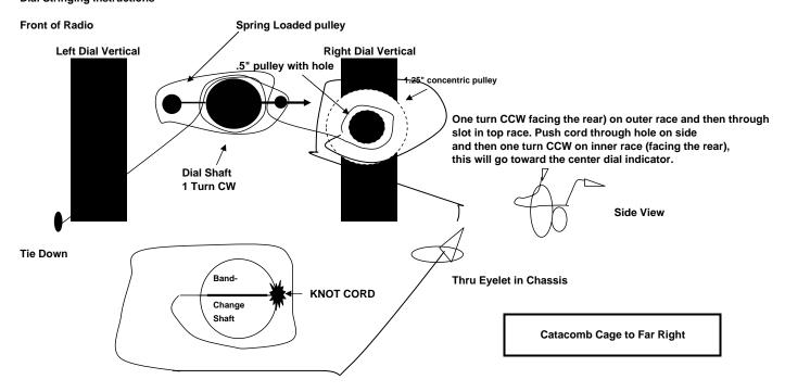
With Catacomb at extreme right side wind 5 turns of cord. .028 diameter cord is just right. CCW around dial shaft
